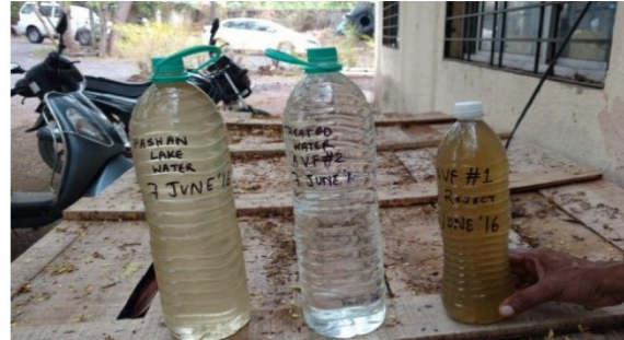
Raw water AVF Treated Water Reject water
